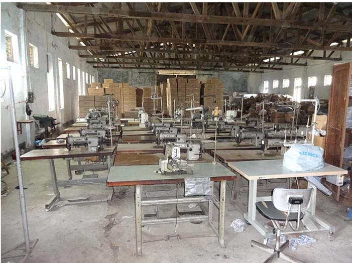
Smart Myanmar along with an international expert from ESGE suggested to develop a servicing schedule to ensure that machines in operation as well as unused machines are maintained at regular intervals. Stored machines are to be covered to protect them and oiled to prevent rust formation and thus, keep them operational and ready for use at any given time. This ensures that the production unit is flexible and fast in replacing defect machines or setting up additional machines.
